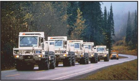
Vibroseis trucks generating seismic reflection data near Stewart, BC during the LITHOPROBE SNORCLE transect
