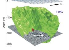
LITHOPROBE Trill 3D seismic reflection image from Sudbury, Ontario. Ore body (red) detected.
